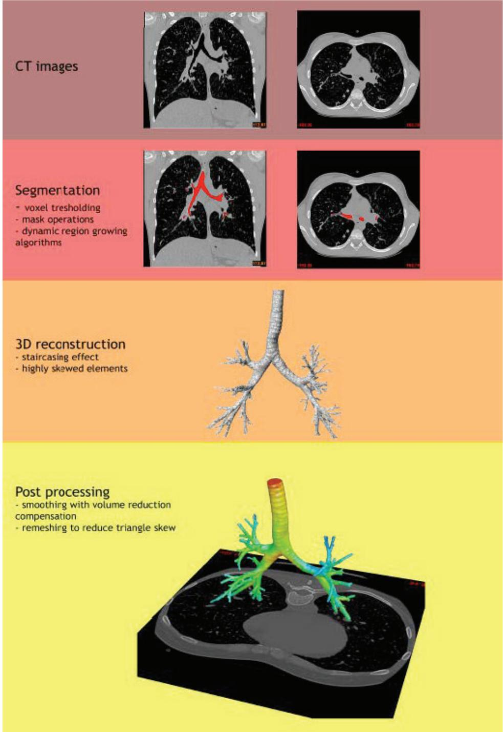
**Figure 2.2.** Segmentation workflow
